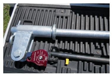
Surface rust does not require immediate removal of the Lite Gin Pole. Rust that has caused pitting, scaling or noticeable visual changes in the steel require the Lite Gin Pole to immediately be removed from service.
